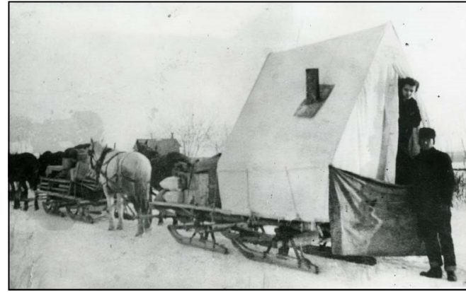
A couple traveling over the Edson Trail by horse and caboose. A caboose was a small canvas covered sleigh which served as shelter and kitchen for the settlers on the long trip, ca. 1911 (SPRA 0024.01.09.07)
